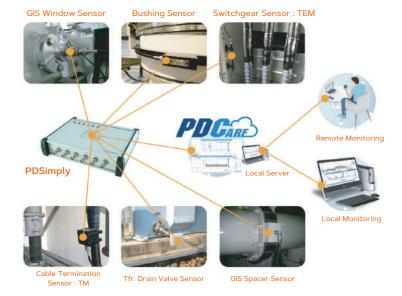
PDSimply is an economical partial discharge monitoring system for continuous on-line monitoring of most HV/MV electrical apparatus. PDSimply continuously acquires and processes data from compatible PD sensors for PD diagnostics.
