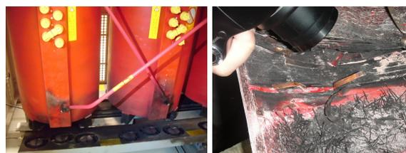
Fig. 2 Insulation breakdown initiated by heat aging (poor connection)
