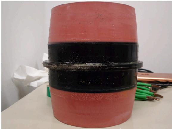
(c) bus socket with defect
