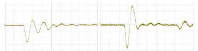
(c)HFCT output with amplifier (d) TM output (50 mV/div, 100 ns/div)
