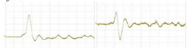
(a) coupling capacitor output (b) UHF output (200 mV/div, 100 ns/div)
