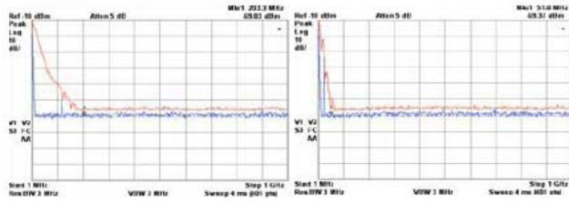
(a) Calibration generator output (b) coupling capacitor output without preamp
