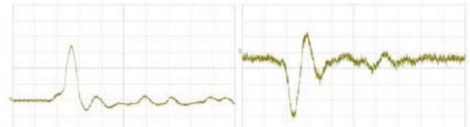
(a) coupling capacitor output (b) HFCT output (200 mV/div, 100 ns/div)
