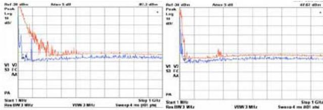
(a) coupling capacitor output (b) TM output with preamp 15 dB with preamp 15 dB
