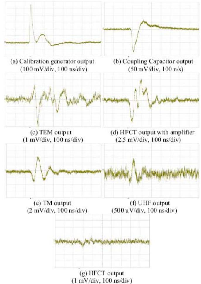
Figure 3 measured waveforms of different sensors at 500 pC apparent charge
