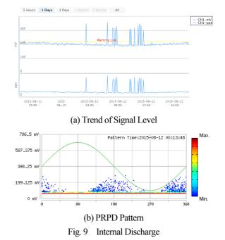
In field, if only PRPD pattern (shown in Fig. 9(b)) is measured, it could be classified as surface discharge or internal discharge, and other measurement should be done to identify the type of discharge. Actually, if the trend of signal level were measured, it would be easily separated from each other.
