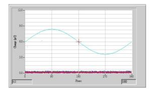
(b) 2nd measurement (2 months later) Fig. 4 PRPD patterns of surface discharge at different dates (continued)
