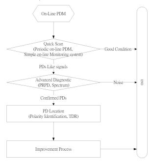
Fig. 1 the flow chart of on-line PDM on MV system
