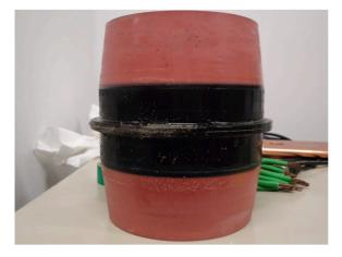
(c) bus socket with defectFig. 6 PD location by TDR (cont.)
