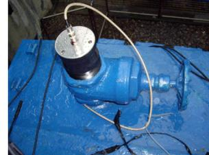
Fig. 13. internal sensor installed in oil valve.
